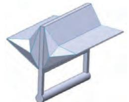
Fig 2. The enclosed origami-inspired WEC design.
