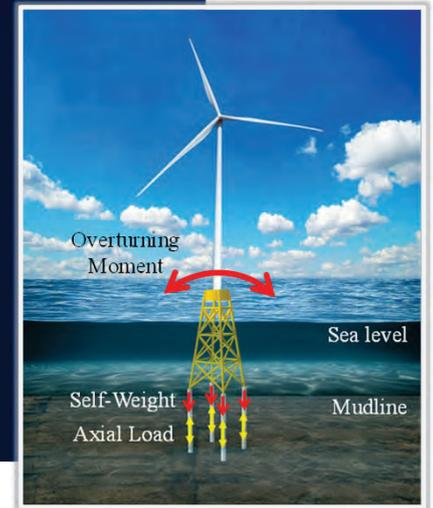
Fig.1 Load transfer in jacket foundations
