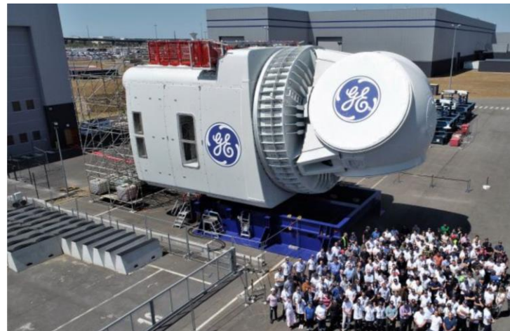
GE 12-MW Wind Turbine Nacelle – Haliade -X
