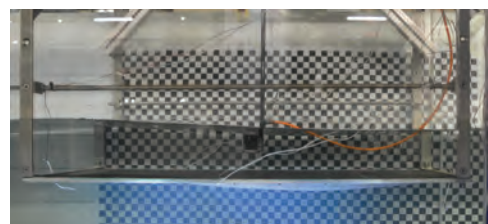
Fig 2. Photograph of neoprene rubber with four-edge fixed frame
